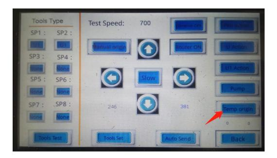
Press "back" to let the the control pannel return to the home page, then machine will cut the material automatically.
